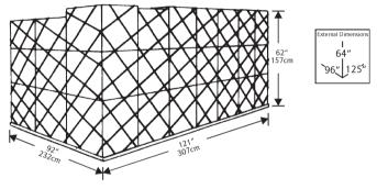
Wide body aircraft. Half width lower deck container. Suitable for the following aircraft: ■ Boeing 767
