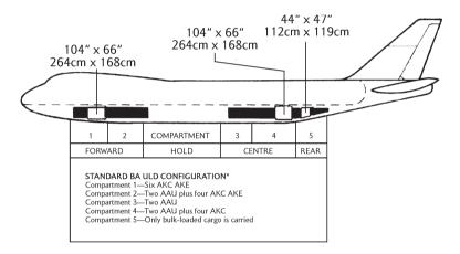
\*The following equipment can be used in place of the 'Standard Configuration' to suit load requirements and to allow interchangeability with other carriers or aircraft.
